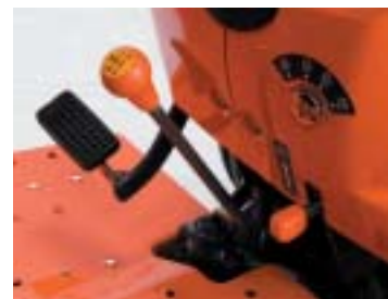
Partially synchronised main gear shift
