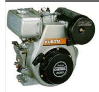
Kubota's advanced engineering technology presents a compact, direct-injection type diesel engine. This lightweight diesel's combustion chamber is placed in a cavity on top of the piston to minimize gas leakage, prevent heat loss and improve fuel economy.
